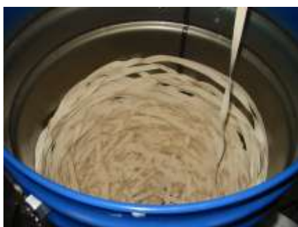
The ribbon will be lay down in a special ton. Through a rotating movement the winding get out of the ribbon.
